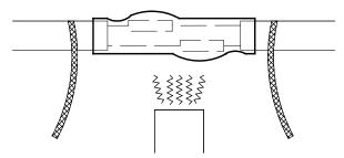
Center the 152mm (6") length shrink tube over the connectors leaving the braid straps exposed. Shrink with heat gun until completely shrunk. A uniform bead of glue should apear around the ends of the shrink tube.
