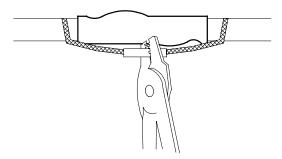
**5** If necessary, cut excess length from braid straps. Crimp the braid straps together into an uninsulated splice connector, then secure the connector at the indented area with one and a half wraps of electricians' tape.
