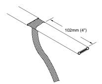
**S** At the bulge, separate the braid to make an opening.
