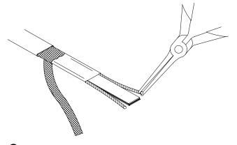
• Starting at the end, pull each bus wire away from the core material.
