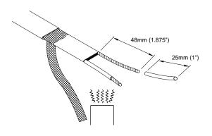
• Slide one 3mm (.125") diameter, 25mm (1") length shrink tube over each bus wire, leaving approximately 13mm (.5") of each bus wire exposed. Shrink with heat gun until completely shrunk.
