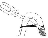
**6** While bending the heater cable, work it through the braid opening.
