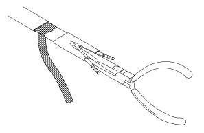
While still warm, spread bus wires and squeeze between them using needle-nose pliers, hold for 5 seconds. Allow power termination to cool before use.
