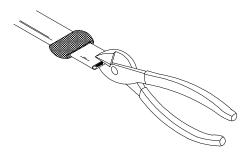
At the end of the heater cable, snip a 9.5mm (.375") slit between the bus wires. Slightly spread wires apart.
