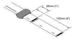
• Cut heater cable off at required length. Strip overjacket back 102mm (4") from the end of heater cable. Slide braid back over the overjacket portion of the heater cable. Cut off excess heater cable leaving 25mm (1").
