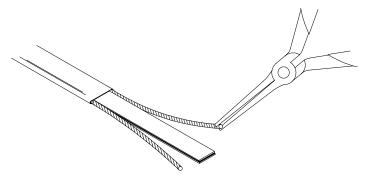
Starting at the end, pull each bus wire away from the core material.
