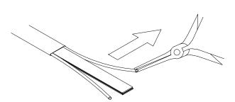
Starting at the end, in the same plane as the cable, pull each bus wire away from the core material.
