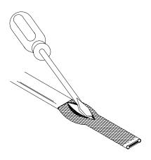
**S** At the bulge, separate the braid to make an opening.
