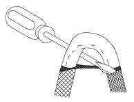
**3** While bending the heater cable, work it through the braid opening.
