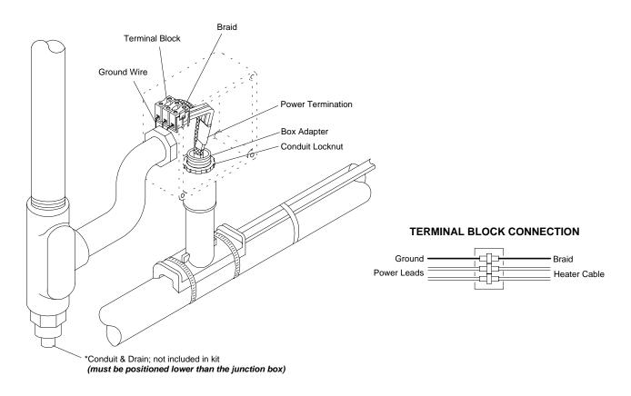
Note: This detail shows internal grounding of braid.
