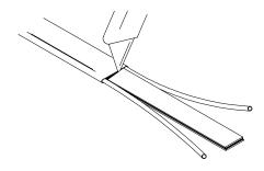
**6** Remove exposed core material.
