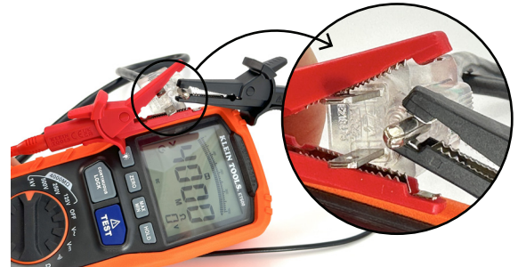
Notes: Set megger to 1000v. Both prongs of plug need to be shorted together during test, as shown above.
