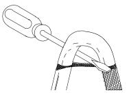
**6** While bending the heater cable, work it through the braid opening.
