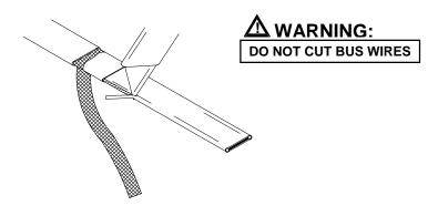
Shave the core material from the outside of each bus wire.
