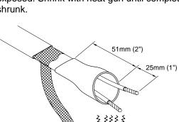
2 Slide one 13mm (0.5") diameter, 51mm (2") length shrink tube over both pigtail leads leaving approximately 25mm (1") of each pigtail lead exposed. Shrink with heat gun until completely shrunk.
