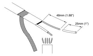
O Slide one 3mm (0.125") diameter, 25mm (1") length shrink tube over each bus wire leaving approximately 13mm (0.5") of each bus wire exposed. Shrink with heat gun until completely shrunk.
