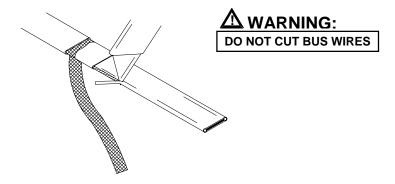
**4** Shave the core material from the outside of each bus wire.
