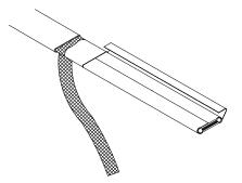
**3** Remove the jacket from the heater cable.
