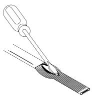
**5** At the bulge, separate the braid to make an opening.
