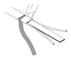
**6** Remove the exposed core material.
