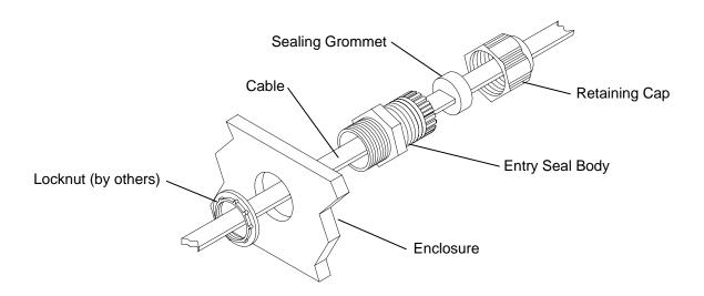
Note: This gland fitting is suitable for use with any approved enclosure with a maximum wall thickness of 4.76mm (.1875") or any enclosure with 3/4"NPT tapped cable entries.
