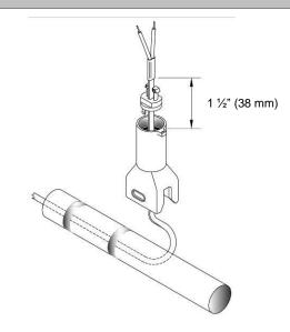
Allow 1 ½" (3.81 cm) of heating cable to remain above top of standoff body.
