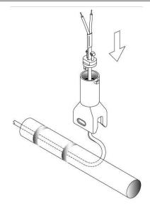
Pull excess heating cable back through standoff.
